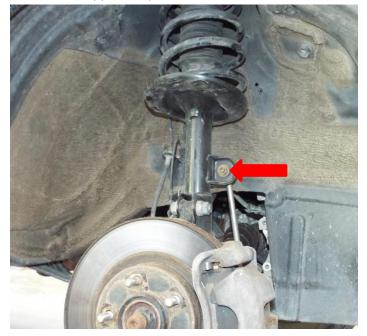
3. Remove the brake line retaining bolt (14mm), and move brake and ABS lines away from the strut body. Using a small screwdriver, open the plastic clip holding the ABS line to the strut body.
