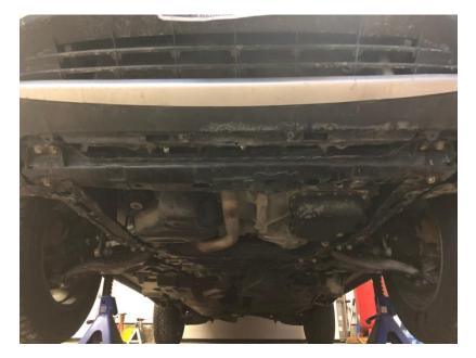
2. Remove two front frame bolts, inboard side, one from each side. Left side shown in pic. 17mm
