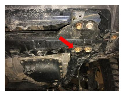
3. Remove two rear frame bolts, one from each side, inboard side. Left side shown in pic.
