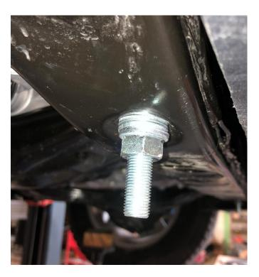
Northwoods Performance skid plate may be installed with or without portions of the factory splash guard. We recommend use of front and engine bay splash guards. Modify and cut the splash guards with a utility knife or cut off wheel.
