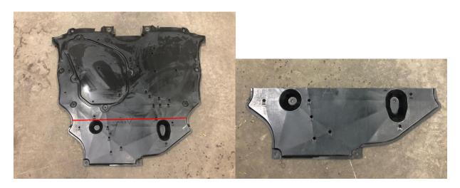
4. Install the front and engine bay splash guard segments using the factory hardware.
