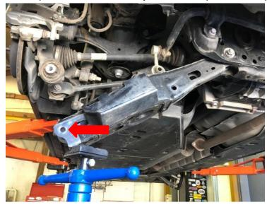
6. Remove the two upper shock mount bolts. 17mm
