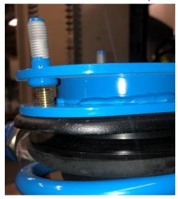
8. Complete spacer installation with the provided nuts and small washers. Use of a thread locking compound is recommended.
