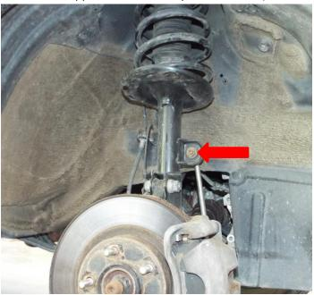
3. Remove the brake line retaining bolt (14mm), remove the ABS line clip from the strut with a screwdriver, and move brake and ABS lines away from the strut body.
