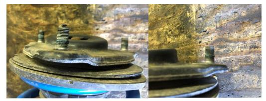
7. Install the Northwoods lift spacer plate on to the strut mount. Verify there is clearance between the strut mount studs and the lift spacer studs.
