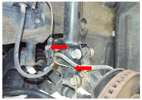
4. Remove the two lower strut nuts and bolts (22mm). Support the lower a-arm and spindle assembly from over extending the drive axle.
