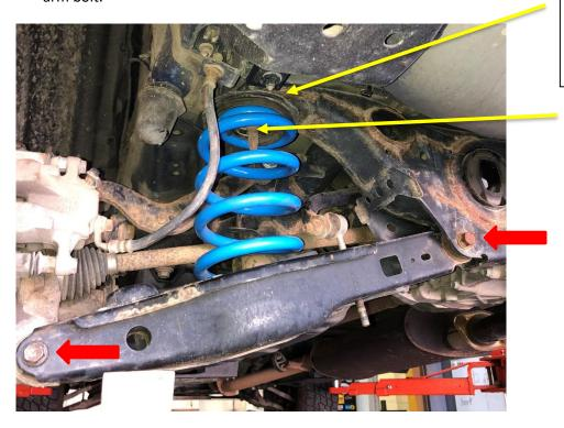
LIFT BUSHING INSTALLS BETWEEN UPPER SPRING PERCH AND REAR SUB FRAME
