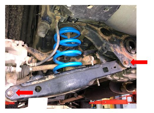
7. Use the jack to slowly lower the control arm until the spring is no longer in compression. Remove the spring.
