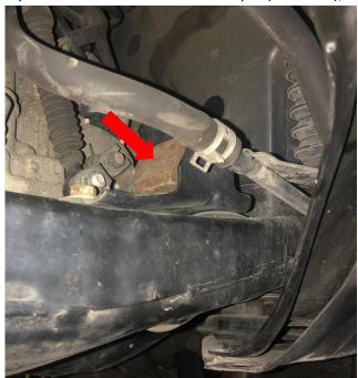
4. Intall the front mounting bolts from the top down on both sides. Installation stack up from the top down will be bolt, small washer, frame member, bushing, flange nut installed with flange facing down. Tighten securely.
