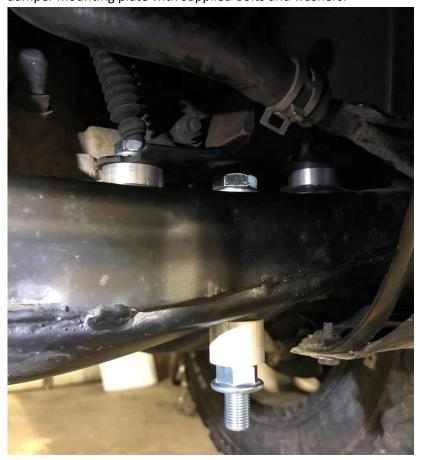
6. Locate the two factory holes, one each side, in subframe members immediately forward of the lower control arm rear mount. Left side of vehicle shown. Holes may have plastic covers installed—remove.
