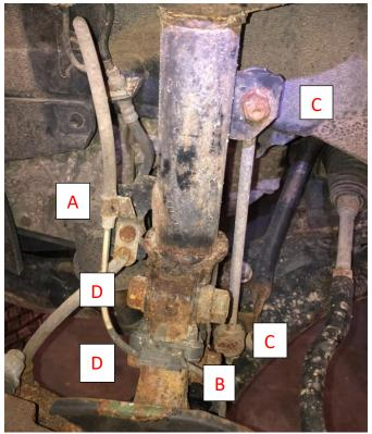
3. Remove the last upper strut body nut and remove the strut.
