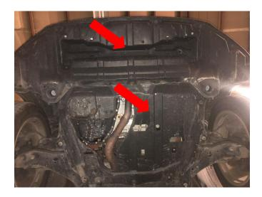
2. Remove the harmonic damper mounted on the left side of the core support cross member.
