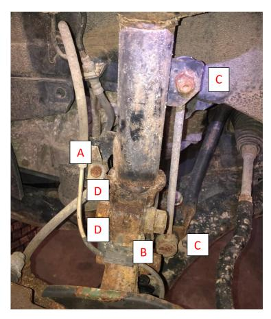
4. Remove the last upper strut body nut and remove the strut.
