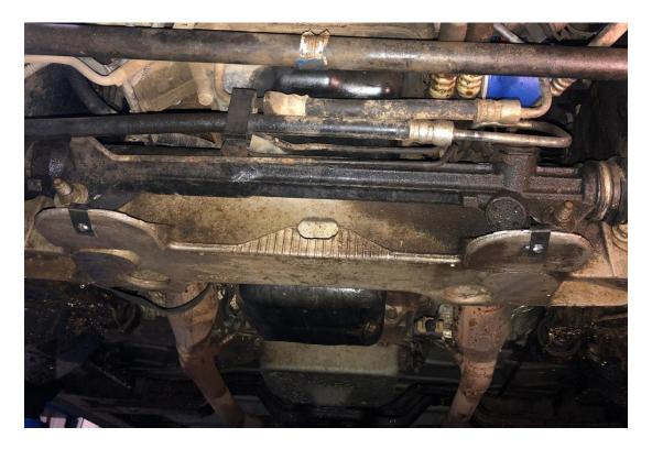
6. Install the skid plate and all hardware. Align the plate, and tighten the front body mounted brackets, the rear skid plate bolts, and the front skid plate bolts.
