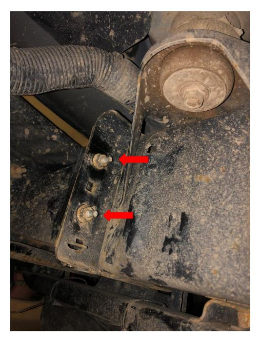
3. Install the front brackets with the flat plate facing forward, using the 5/16 hardware. Install the bolts loosely—do not tighten until skid plate is fully fitted.
