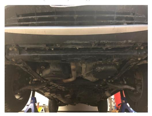
2. Remove two front frame bolts, inboard side, one from each side. Left side shown in pic. 17mm
