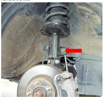
3. Remove the brake line retaining bolt (14mm), and move brake and ABS lines away from the strut body. Using a small screwdriver, open the plastic clip holding the ABS line to the strut body.
