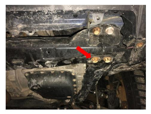
3. Remove two rear frame bolts, one from each side, outboard side. Left side shown in pic.
