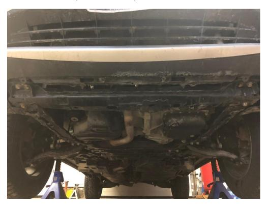
2. Remove the two front flange bolts and springs. Save for re-use. (modified pipe shown above)
