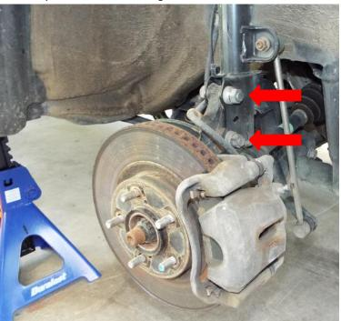
5. Remove the final strut top retainer nut and remove the strut assembly.
